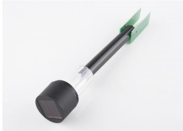
In this tutorial, we are going to take a simple solar powered pathway light from a department store and rewire it to be a soil moisture sensor. The finished design will turn on an LED when the soil dries up.
