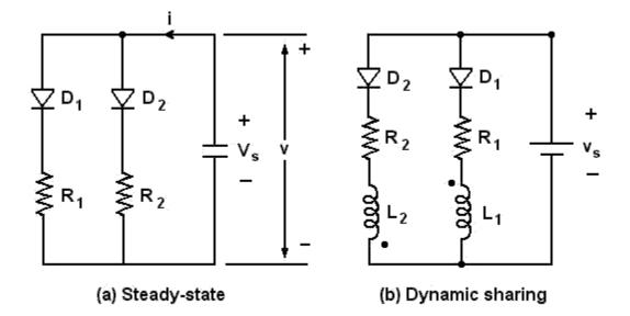
Diodes of same type having same voltage drops can be used for steady state conditions. In this case, the parallel diodes would have the same reverse blocking voltages. Some precautions are to be kept in mind while using the diodes with same forward voltage drops, which are:
