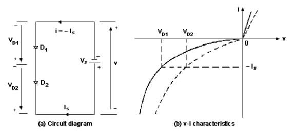
V-I characteristics show that the diodes have different blocking voltages. In forward biased state, the voltage drop and the forward current would be same on the diodes. While in the reverse biased the blocking voltage is different as the diodes have to carry the same leakage current.
