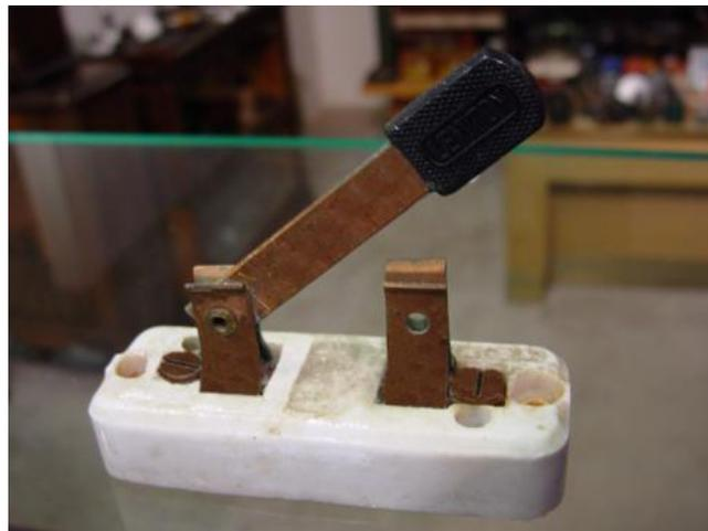
A knife switch is nothing more than a conductive lever, free to pivot on a hinge, coming into physical contact with one or more stationary contact points which are also conductive. The switch shown in
