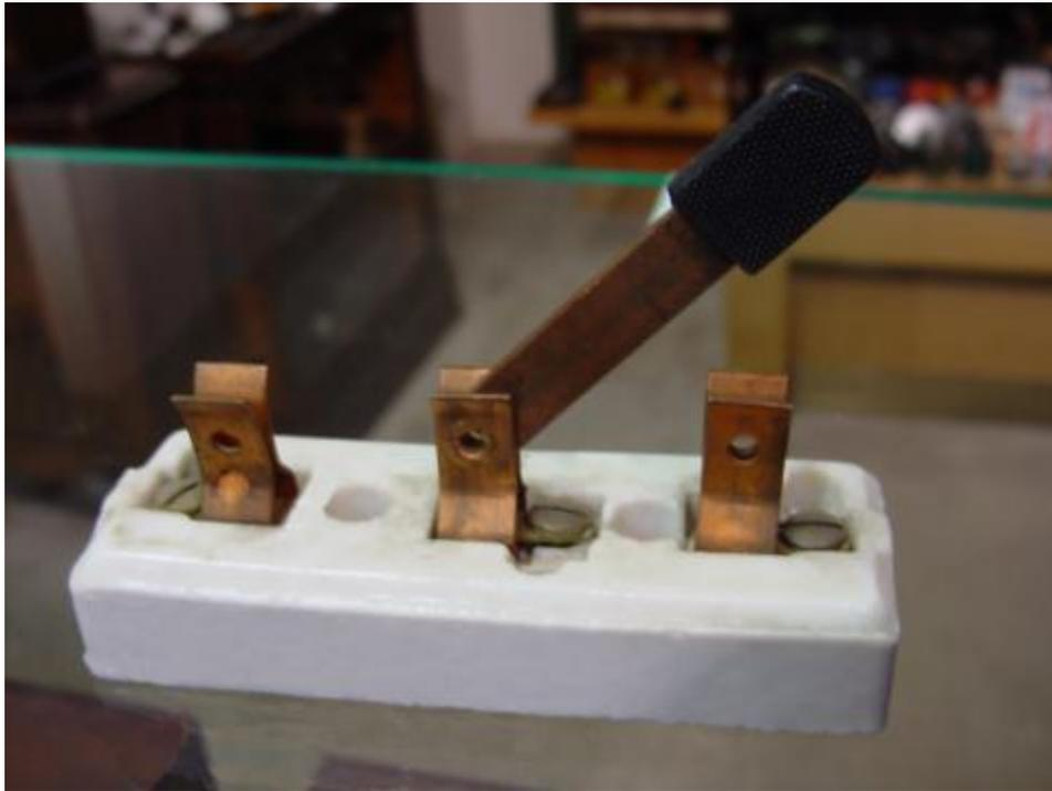
The particular knife switch shown here has one "blade" but two stationary contacts, meaning that it can make or break more than one circuit. For now this is not terribly important to be aware of, just the basic concept of what a switch is and how it works.
