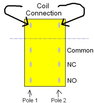
This is the schematic symbol for a DPDT relay. Schematic drawings are not currently discussed on this website but this schematic helps to understand the connections to a relay. The block on the left side represents the coils and the two wires extending up and down are the coil connections. When no power is applied to the coil the common connection is connected to the normally closed connection. When
