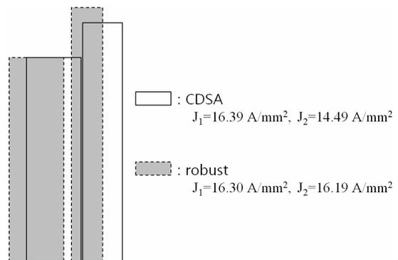
**Fig. 4.** Comparison of two SMES magnet designs after optimization
