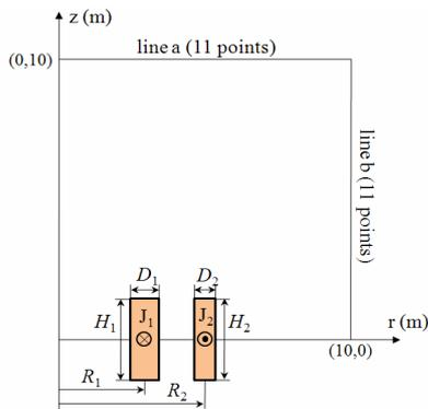
**Fig. 3.** Configuration of the SMES with eight design variables
