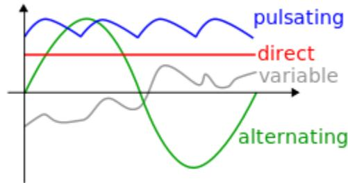
Direct Current (red curve). The horizontal axis measures time; the vertical, current or voltage.
