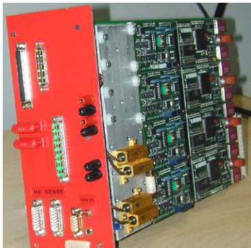
Figure 1: The Test Fixture developed by Torino-INFN and CAEN for the quality control on A4601H production
