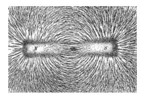
Magnetic field lines emanate primarily from the north pole of a magnet and curve around to the south pole. They can be revealed by scattering iron filings on a piece of paper over a magnet.
