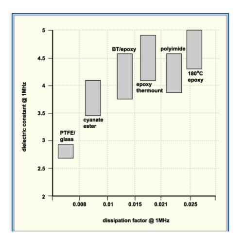
The most common high-frequency materials are made from PTFE mechanically reinforced by glass fibre to improve mechanical stability and reduce cold flow of the material. However, woven reinforcements tend to produce anisotropic dielectric properties, so randomly distributed short micro-fibres are used to give better results. Improved dimensional stability and thermal conductivity is sought by adding ceramic fillers to the micro-fibre reinforcement.
