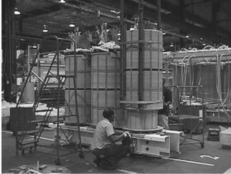
Figure 2 - Concentric arrangement, outer coil being lowered onto core leg over top of inner coil
