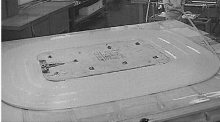
Figure 6 - Pancake winding during winding process
