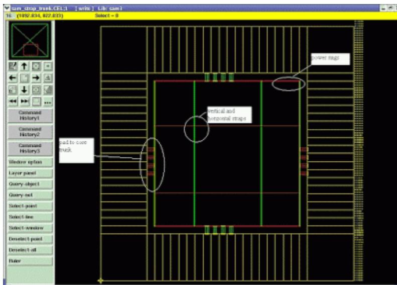
Figure (2) Showing core power ring, Straps and Trunks
