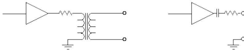
The triangles represent amplifiers or some other source of current. There's always some combination of resistors, capacitors and /or transformers to adjust the output voltage and protect the current source from short circuits. Whatever is after the current source is going to have impedance– it's usually all lumped together and called the "source impedance".
