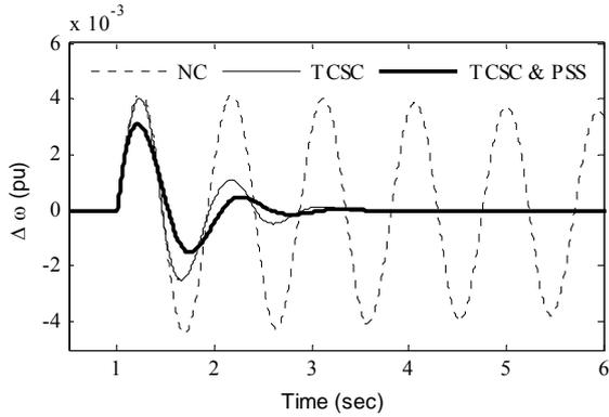
Fig. 19 Variation of speed deviation  $\Delta\omega$  : Case-2
