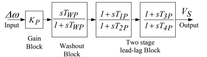
Fig. 3 Structure of the power system stabilizer
