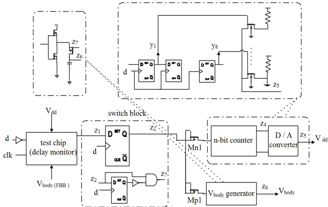
Fig. 2 Expanded proposed  $V_{DD}/V_{TH}$  monitoring circuit
