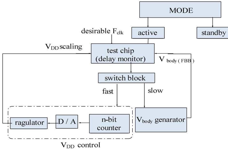
Fig. 1 Diagram of proposed design for active mode
