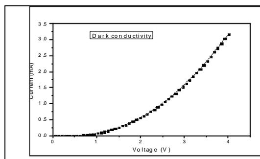
Figure 3: Dark Characteristics of Organic Solar Cell.
