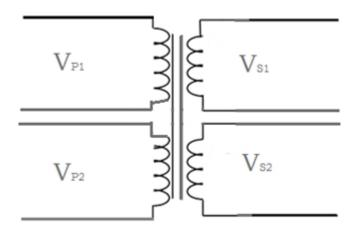
So each secondary coil produces the amount of voltage which is directly proportional to its number of turns, since all the coils are electrically isolated and magnetically linked to each other, and to the primary coil as well.
