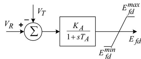
Fig. 2 Simplified IEEE type ST 1A excitation system
