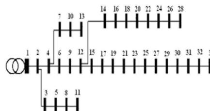
Fig. 2- 33 bus power distribution system Ref. [16]
