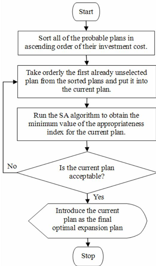
Fig. 2. The flowchart of the proposed planning procedure.
