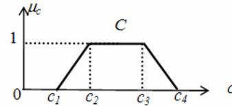
Fig. 3. Typical membership function of an input variable.
