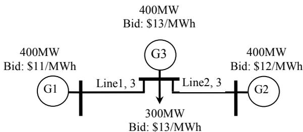
Fig. 1. The 3-bus example power system
