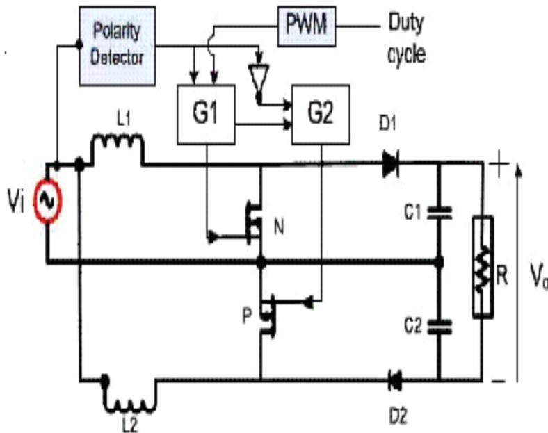
Figure 2 System for dual boost power converter
