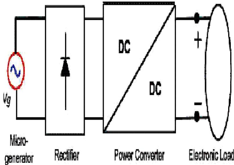
**Figure.1: Block diagram of two stage power converter**
