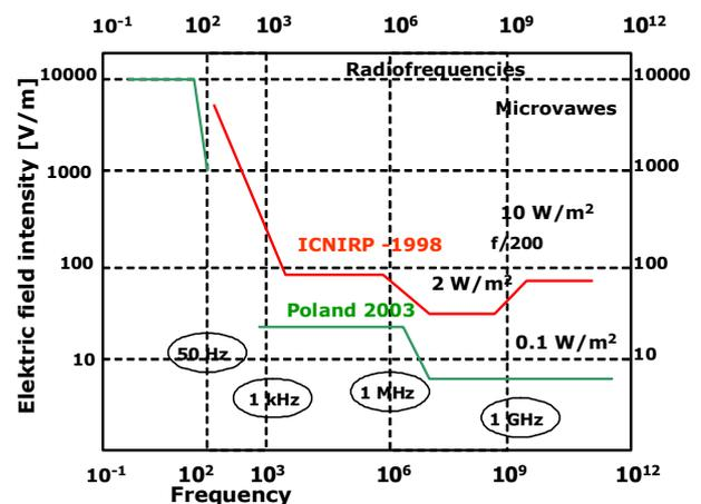
Fig. 1 Permissible public exposure levels in electric field
