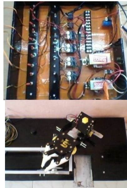
Fig. 3 : Relay Panel And Conveyor With Robotic Arm
