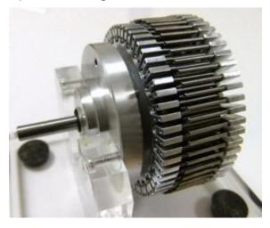
I took a liking to this motor on a recent review I was doing on new Electric motor technology. Although 100 watts and 200 grams weight may not sound impressive, it is when you need power for robotics and other specialist uses the power to weight ratio is important. This is also important for electric vehicle applications where weight is critical. Existing small motors are less than 200 watts per kilogram.
