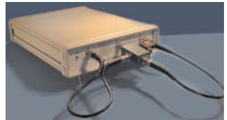
Figure 4: Impedance measurement test setup using the AP200 frequency response analyzer.
