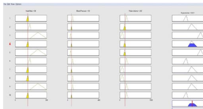
Fig. 5. Rules viewer window of FLMS-2 with 10 different rules and rule number four is executed to alert the moderate hypovolaemia
