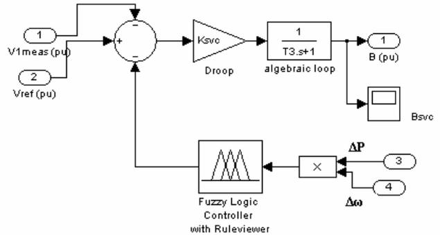
Fig.5 SIMULINK model of FLC controller for SVC
