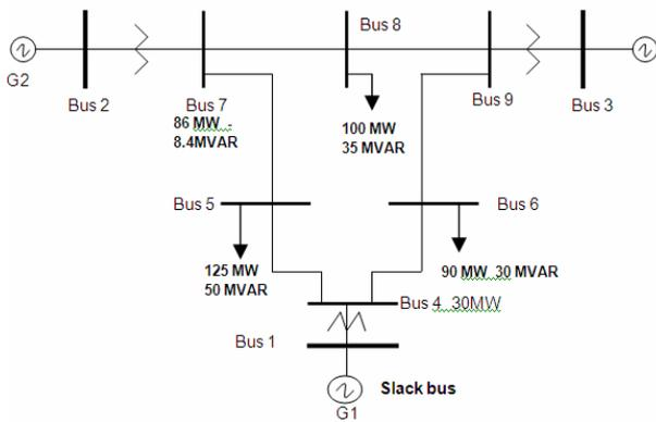
Fig. 8 One line diagram of WSCC system
