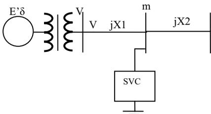
Fig.4 SMIB system with SVC - single line diagram
