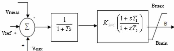
Fig.1 Block representation of SVC control
