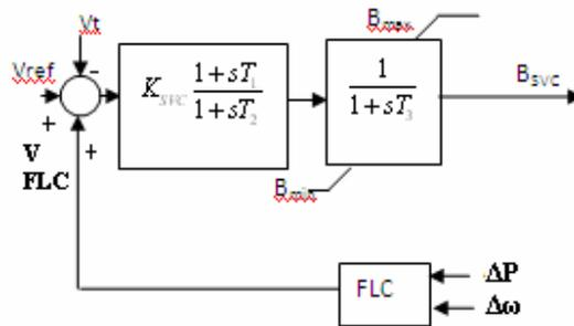
Fig. 2 Block diagram of proposed Fuzzy logic controller
