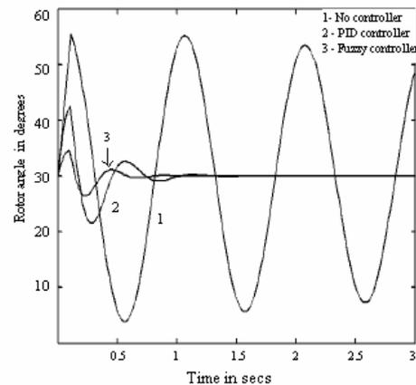
Fig.6 Variation in rotor angle for different controllers of SVC
