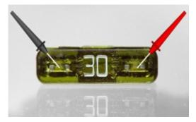
In order to check the fuse, a probe is used with readings from the terminals. The correct functioning would be when the value is 0V DC. The fuse should be checked with the voltage being supplied.
