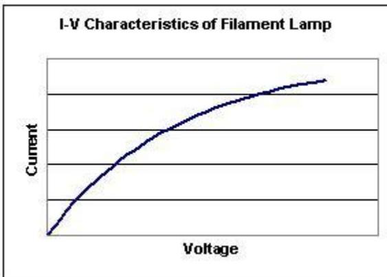
As the voltage across the filament lamp increases the current increases, but it does not do so linearly. You need to know this and be able to sketch this graph for the IB exam!
