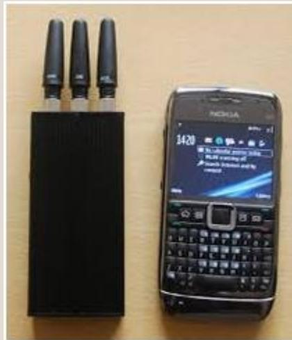
Jamming may be used for radio signals, mobile phone signals or radar signals. In a war the aims is simply cutting the communication through the air of the opponent and make them lose control of the war. Here the tricky point is adjusting your frequency with the opponent's frequency so that you can give enough power to the jammer that suppresses that frequency.
