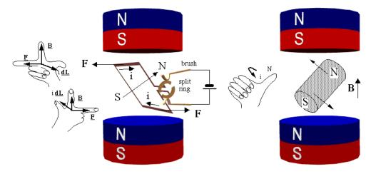
The force F on a wire of length L carrying a current i in a magnetic field B is iLB times the sine of the angle between B and i, which would be 90° if the field were uniformly vertical. The direction of F comes from the right hand rule\*, as shown here. The two forces shown here are equal and opposite, but they are displaced vertically, so they exert a torque. (The forces on the other two sides of the coil act along the same line and so exert no torque.)
