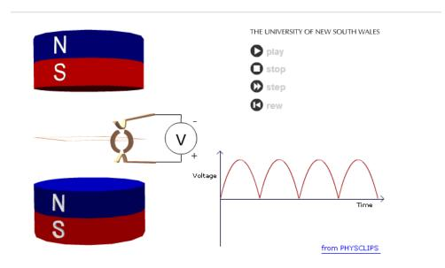
If you use mechanical energy to rotate the coil (N turns, area A) at uniform angular velocity  $\omega$  in the magnetic field **B**, it will produce a sinusoidal emf in the coil. emf (an emf or electromotive force is almost the same thing as a voltage). Let  $\theta$  be the angle between **B** and the normal to the coil, so the magnetic flux  $\varphi$  is NAB.cos  $\theta$ . Faraday's law gives:
