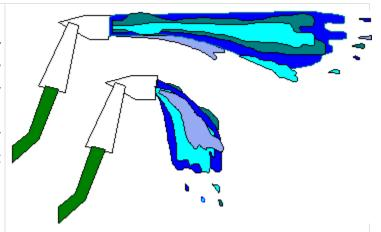
The amount of water exiting each nozzle is the same. However, the water pressure is different.
