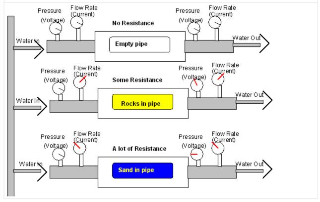
In the empty water pipe there is little resistance so the water pressure (voltage) and water flow rate (current) are the same on each side. With rocks in the pipe there is some resistance to the flow of water and the water pressure (voltage) and the water flow rate (current) are less. With sand in the pipe there is a lot of resistance to the flow of water and the water pressure (voltage) and water flow rate (current) are reduced even further.
