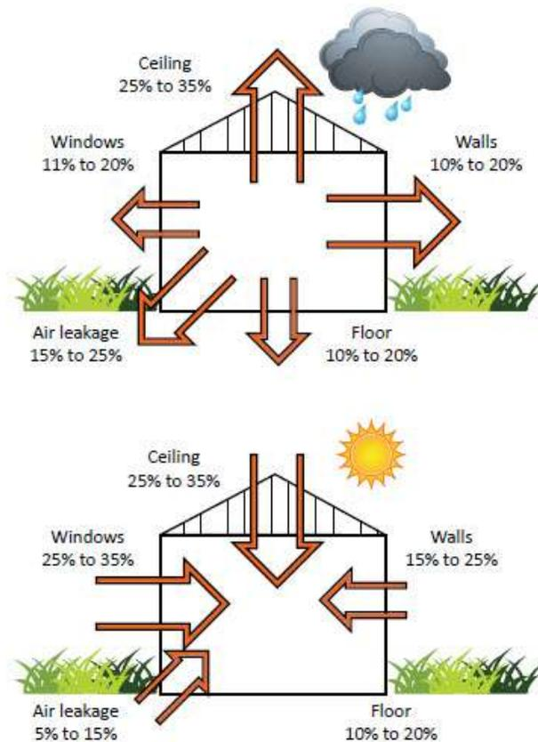
**FIGURE 3.1 Heat flow in an uninsulated cool-climate house.**
