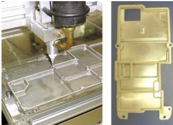
Figure 4. Form-in-Place and Mold-in-Place
