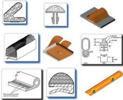
Figure 2. Mounting methods.
