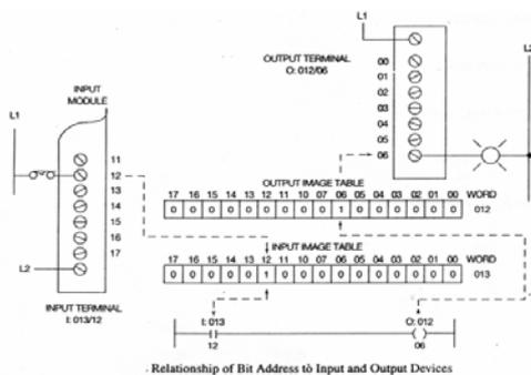
Fig. 1, I/O Pin Configuration of AB PLC
