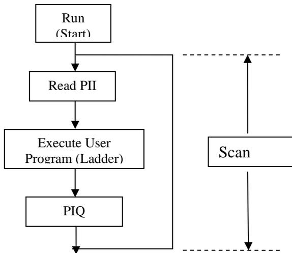
I/O driver (SCADA) picks up PII and PIQ and transfers the image to database and this image is called driver image. This driver image available in SCADA database is used for graphical view of process monitoring from operator station (OS) in the central control room.
