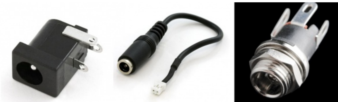
A comparison of three different methods of mounting the same barrel connector: (left to right) board mount, inline cable mount, and panel mount.
