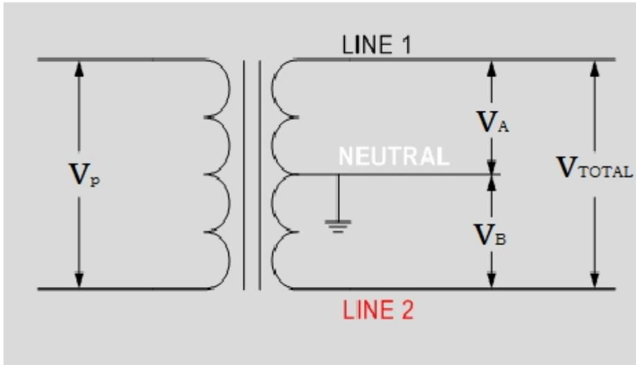
As it can be seen from the figure that this type of configurations gives us two phases through the two parts of the secondary coil, and a total of three wires, in which the middle one, the center tapped wire is the neutral one. So this center tapped configuration is also known as a two phase- three wire transformer system.
