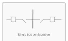
Maintenance of the bus would require the outage of the total system, use of standby generation, or switching to adjacent station, if available. Since the single bus arrangement is low in reliability, it is not recommended for heavily loaded substations or substations having a high availability requirement.
