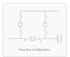
service by tripping the breaker, then opening its isolation switches. Since the other breakers adjacent to the breaker being maintained are in service, they will continue to supply the circuits. In order to gain the highest reliability with a ring bus scheme, load and source circuits should be alternated when connecting to the scheme.
