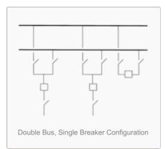
With two buses and a bus tie available, there is some ease in doing maintenance, but maintenance on line breakers and switches would still require outside the substation switching to avoid outages.
