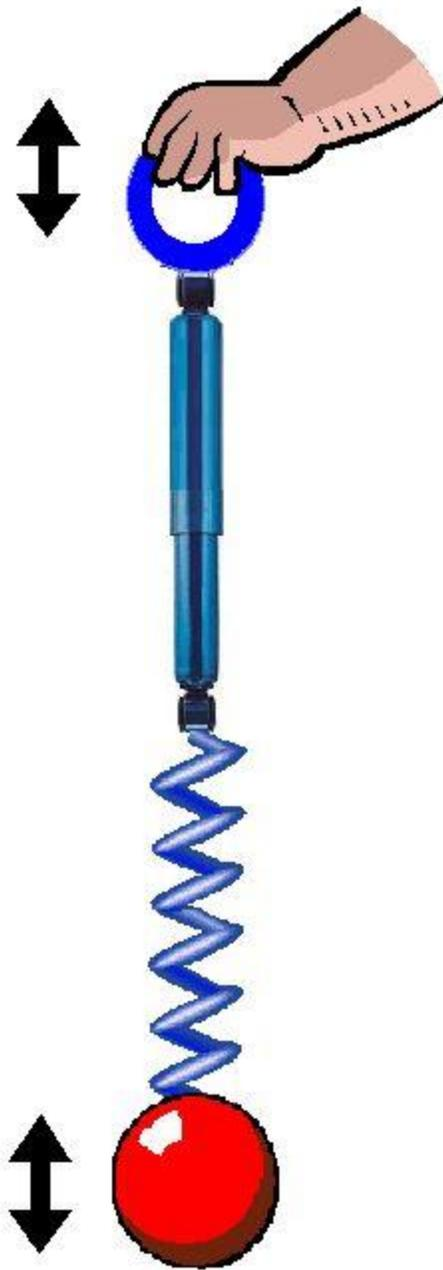
Doing so would certainly achieve the desired objective, but if this were an industrial positioning system, the inordinate amount of time required to move the weight slowly to its final height would degrade the performance of any process that depends on the weight's position. The longer the weight remains above or below the setpoint, the poorer the performance.
