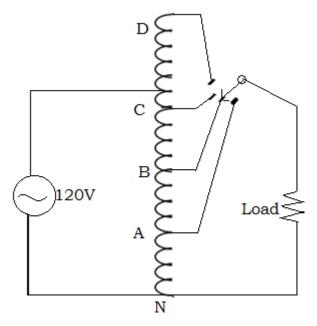
Here it can be seen that there is only a single winding, on which a number of points have been marked, and each point has equal number of turns, i.e. 40 turns between two consecutive points on the winding, which means 40 volts between those two points.
