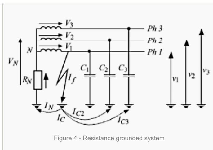
Figure 4 - Resistance grounded system
