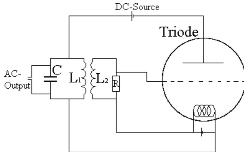
A simple DC to AC converter using 2 solenoids, a capacitor and a triode
