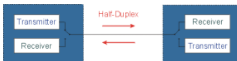
Figure 2 - Half Duplex Communications
