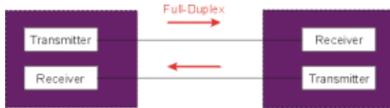
Figure 3 - Full Duplex Communications
