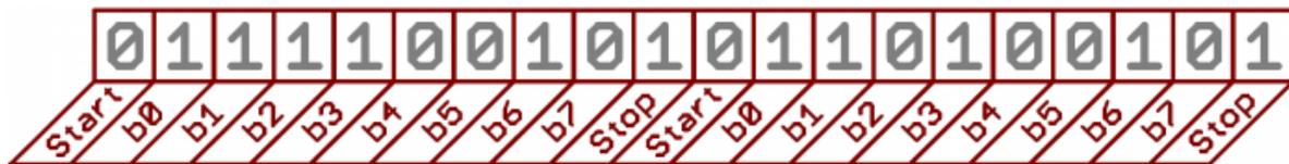
Since we're transferring at 9600 bps, the time spent holding each of those bits high or low is  $1/(9600 \text{ bps})$  or 104  $\mu\text{s}$  per bit.
