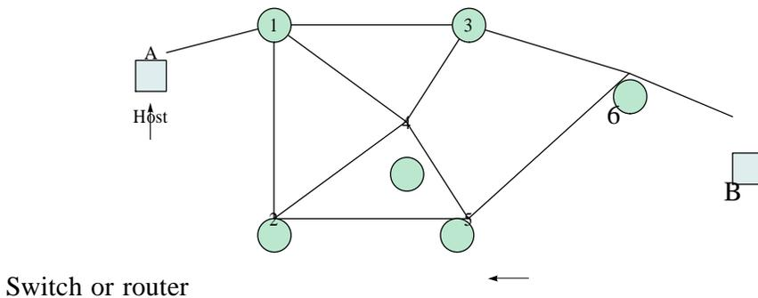
**FIGURE 1.23** An example of a packet-switch network
