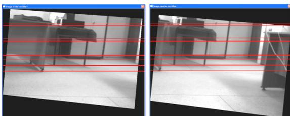
Figure 4. Left and right images obtained after the rectification step.
