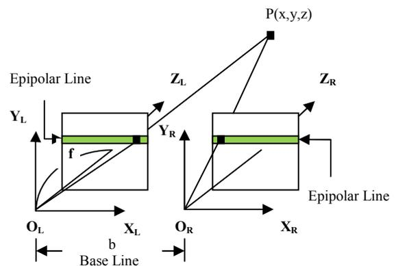
Figure 1. The parallel configuration in stereo vision.
