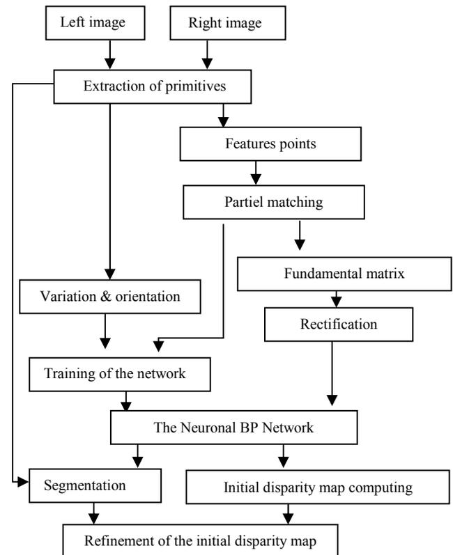
Figure 2. Block diagram of the overall process.
