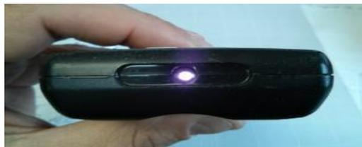
*When the LED is modulating at 38kHz, the LED should appear constantly lit, but dim.*
