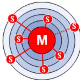
In reality, at a given moment, the master device can only be connected to a single slave at once. Therefore, it quickly switches between slaves in order to make it seem as if it is simultaneously connected to all the slave devices.
