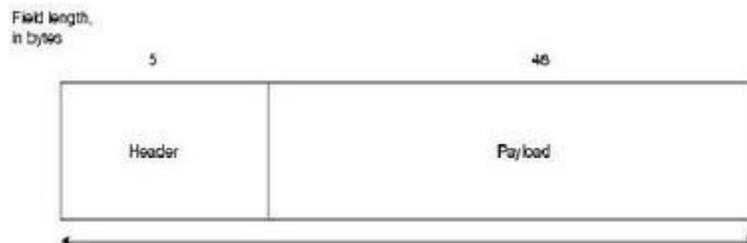
ATM Cell Basic Format ATM transfers information in fixed-size units called cells. Each cell consists of 53 octets, or bytes. The first 5 bytes contain cell-header information, and the remaining 48 contain the payload (user information).
