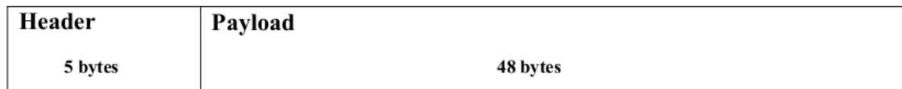
*Fig:ATM cell Format*
