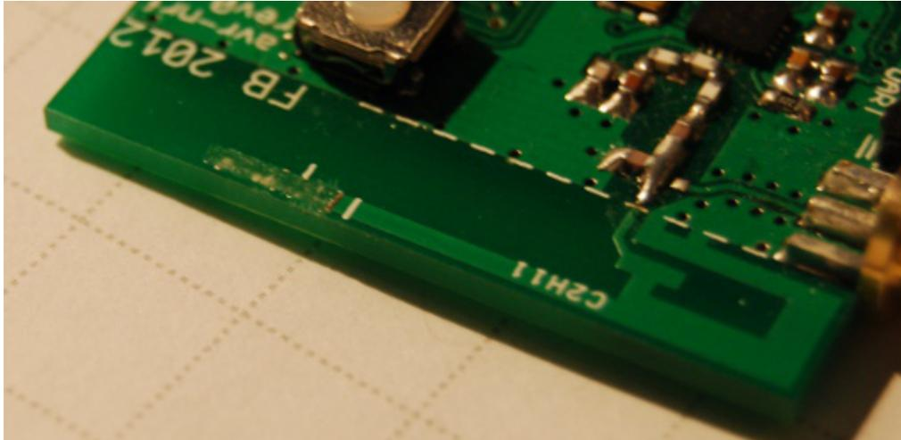
That's how the cut antenna looks like. You can see from the picture that the layout provide a path from the antenna feed point to an RP-SMA connector, used for tuning.
